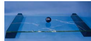
Laminated safety glass made of 2 x heat strengthened glass – both panes broken
