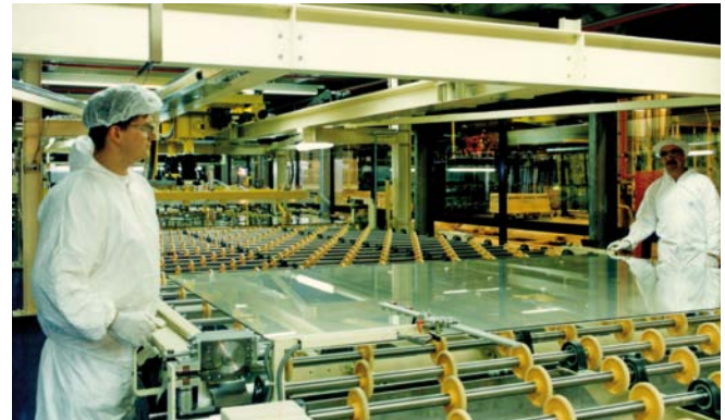
Production of laminated safety glass – clean room
