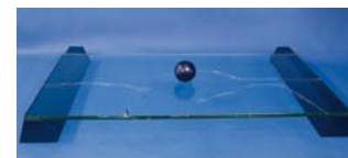
Laminated safety glass made of 2 x heat strengthened glass – top pane broken
